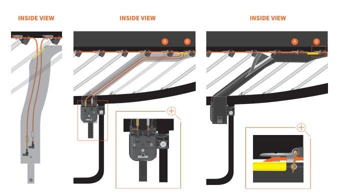
**NOTE** - Cable A with the yellow tag must be plugged into socket A and cable B with the white tag into socket B. The cable plugs and controller sockets are 'keyed' (ie, they will only fit correctly in one position). Line up the green post in the cable plug with the slot in the controller socket. Do not force the plug into the socket; when you have correctly keyed them they will slide together easily.
